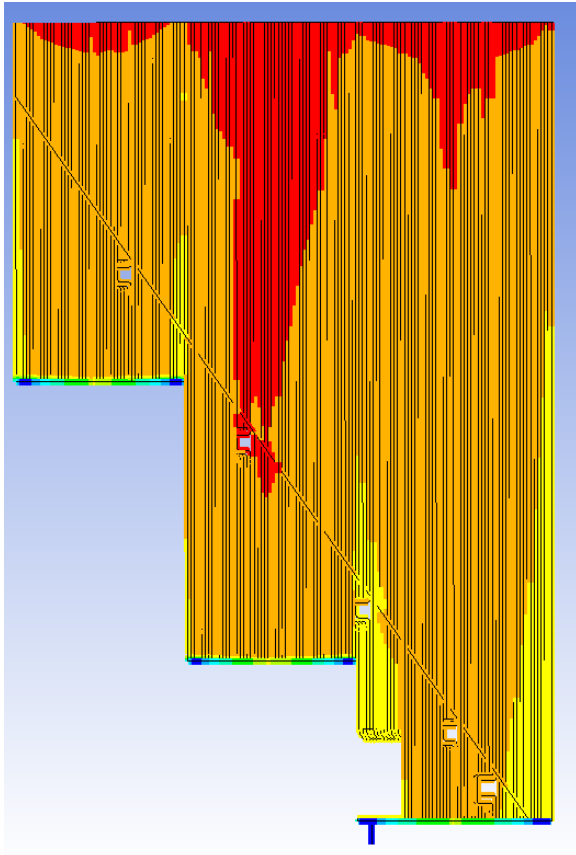
Figure 7: Solved thermal field in Flownex (Front Wall)
